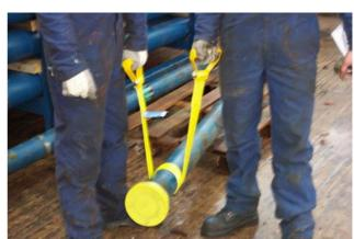
Note: "LIFT-Mate" products are designed for MANUAL handling purposes ONLY and must NEVER be used as part of any mechanical rigging or lifting set up.
